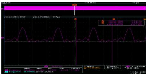
Fig. 4. DDS output as sinc wave obtained on CRO
